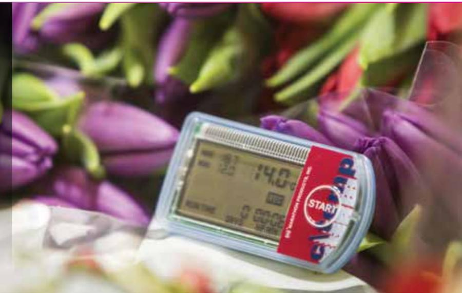
The EDL-4S is our newest addition to the logger range. It measures temperature, relative air humidity, CO2 and vibrations.
